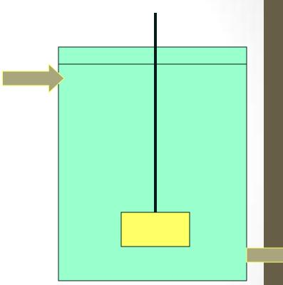
Continuous flow stirred reactor with ultrafiltration-
