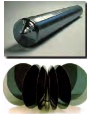
Figure 2.3 Single-crystal ingot and sliced wafers (from [Fullman99]).
