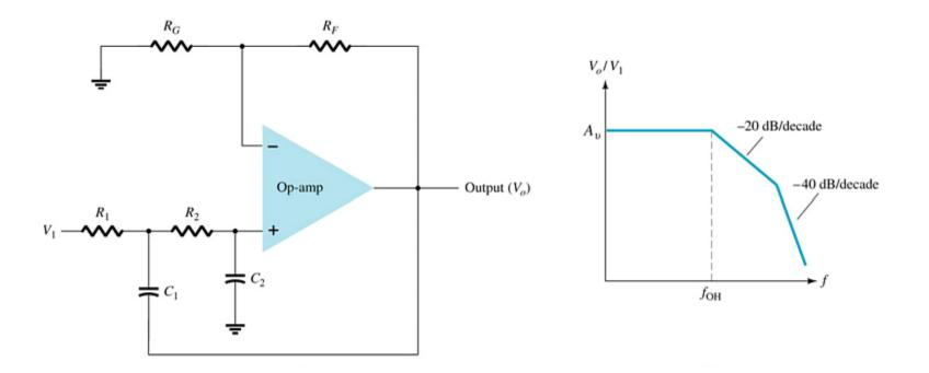
The roll-off can be made steeper by adding more RC networks.
