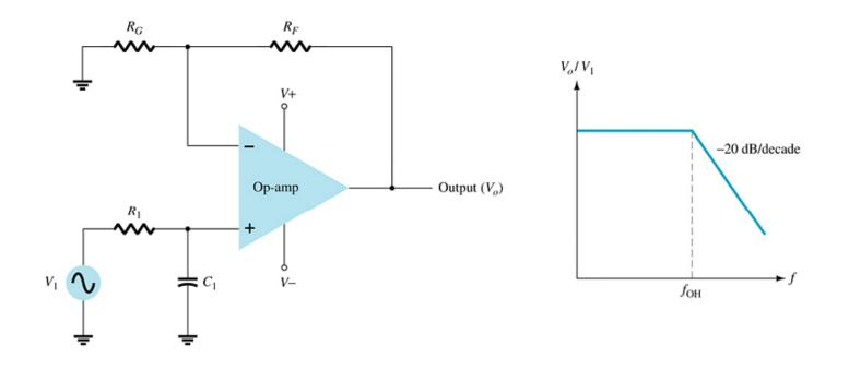
The upper cutoff frequency and voltage gain are given by:
