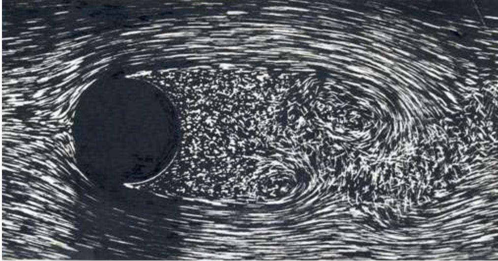
Fig 31.5 (a) Flow Past a Cylinder at Re=2000 [Photograph courtesy Werle and Gallon (ONERA)]
