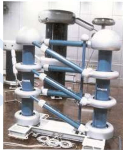
Single metallic body (DC Generator 900 kV)
