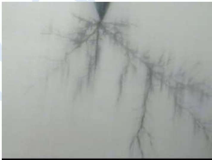
Fig 19.2 Development of Treeing Process in Epoxy Resin
