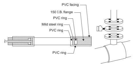
Fig. 1.74 Capacitance type flow/no-flow switch
