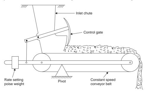
Fig. 1.66 Early belt-type mechanical gravimetric feeder
