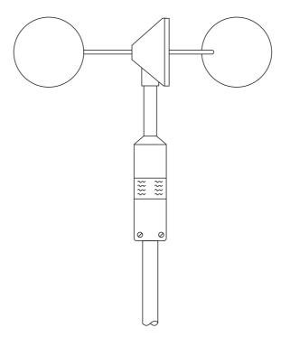
Fig. 1.81 Three cup-anemometer.
