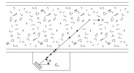
Fig. 1.59 Doppler Flow meter Principle of operation
