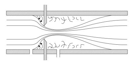
Fig. 1.3 Flow pattern with orifice plate
