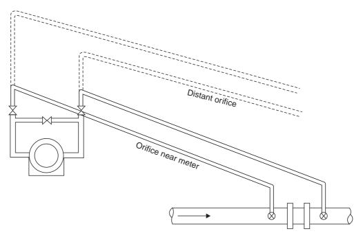
Fig. 1.16 Pressure connections to meter above orifice for air and gases
