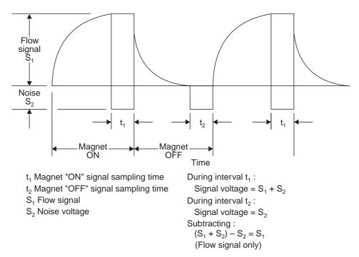
Fig. 1.54 Plot of the output signal
