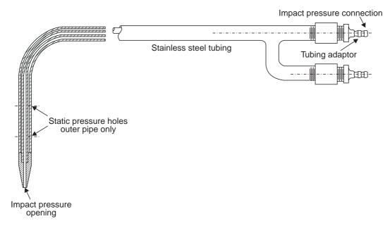
Fig. 1.22 Typical pitot tube
