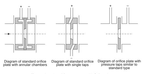
Fig. 1.6 Location of Pressure taps with Orifice plate
