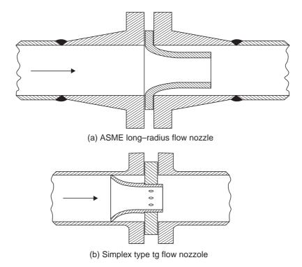
Fig. 1.11 (a) The ASME long-radius (b) The Simplex type tg
