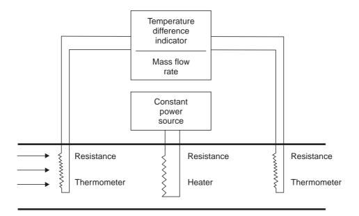
Fig. 1.45 Heat transfer flow meter
