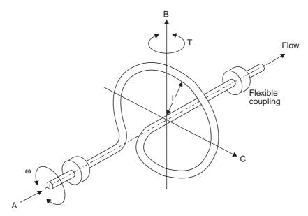
Fig. 1.42 Gyroscopic Mass Flow meter
