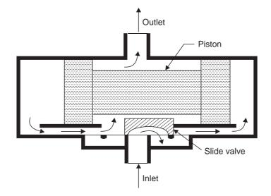
Fig. 1.29 Operating Principle of the Piston meter
