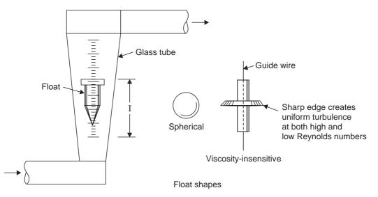
Fig. 1.36 Fundamental operation of a variable area flow meter
