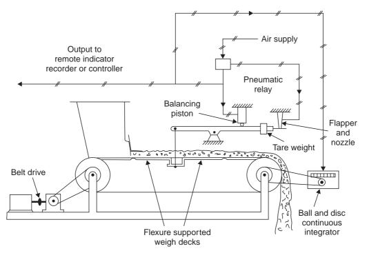
Fig. 1.68 Belt-type gravimetric meter with pneumatic system
