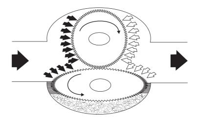
Fig. 1.30 Oval-gear flow meter
