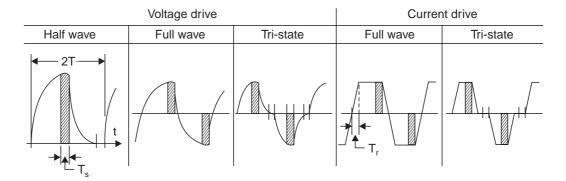
Fig. 1.53 Types of pulsed DC Coil excitation
