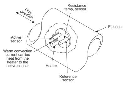
Fig. 1.75 Thermal flow switch
