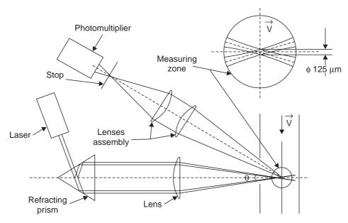
Fig. 1.61 Operation of the laser Doppler anemometer
