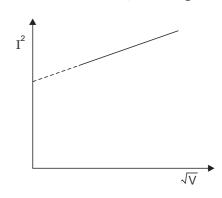
as a function of the voltage  $\sqrt{V}$  is shown in Fig. 1.79. Fig. 1.79 Variation of I<sup>2</sup> with respect to  $\sqrt{V}$  It is called as calibration curve.
