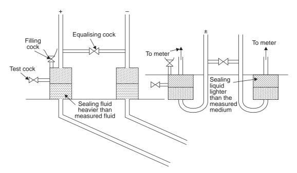
Fig. 1.18 Installation of Sealing pots
