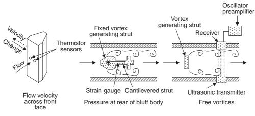
Fig. 1.71 Solid state vortex flow meter detectors
