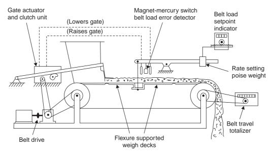
Fig. 1.67 Belt-type electromechanical gravimetric feeder
