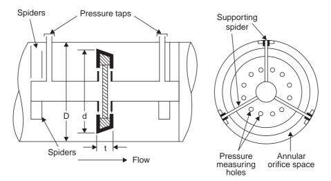
Fig. 1.39 Annular orifice plate installation
