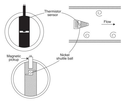
Fig. 1.70 Early vortex flow meter detectors
