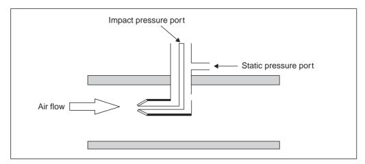
Fig. 1.21 A common industrial type pitot tube
