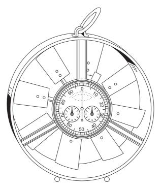
Fig. 1.80 Vane design anemometer
