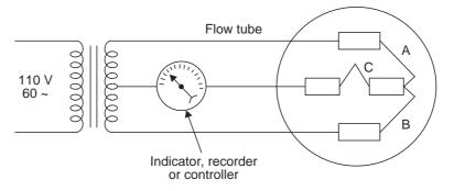
Fig. 1.49 Hot wire flow-sensing probe
