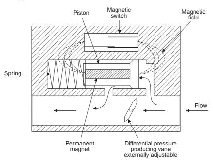
Fig. 1.76 Bypass flow switch
