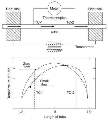
Fig. 1.47 Heated tube-type mass flow meter
