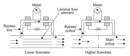
Fig. 1.48 Bypass-type thermal mass flow meters
