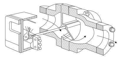
Fig. 1.73 Swinging vane flow switch
