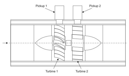
Fig. 1.41 Twin-turbine mass flow meter
