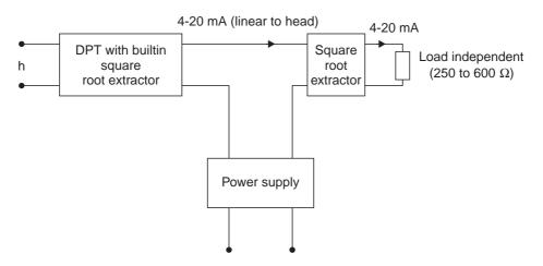
Fig. 1.26 Differential Pressure transmitter with external square root extractor.
