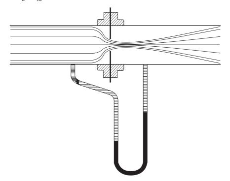
Fig. 1.2 Orifice and Pressure-Differential Measurement
