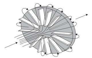
Fig. 1.44 Classical Coriolis mass flow meter
