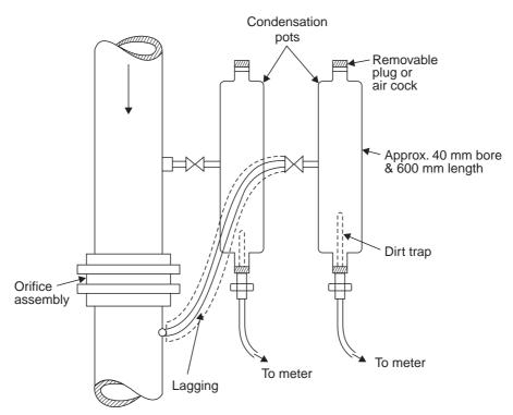
Fig. 1.17 Installation of Condensation pots
