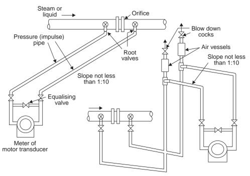
Fig. 1.13 Pressure connections to meter below orifice for liquids and steam
