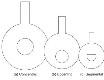
Fig. 1.4 Sketch of orifices of different types
