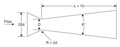
Fig. 1.89 Standard sonic venturi-nozzle
