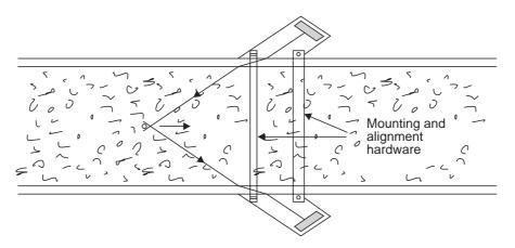
Fig. 1.60 Two-transducer approach
