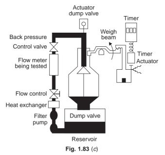
As the weigh tank fills, the weigh pan rises, tripping the timer actuator, and the electronic timer begins counting in milliseconds, starting the actual weighing cycle. The preliminary fill balanced out by the tare weight before actual weighing begins, permits a net measurement of
