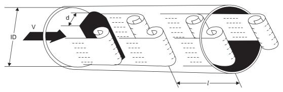
The distance between the Karman vortices (I) is only a function of the width of the obstruction (d) and therefore the number of vortices per unit of time gives flow velocity (V).
