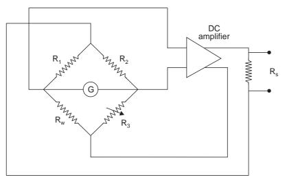
Fig. 1.78 (b) Measuring circuit of a constant temperature type
