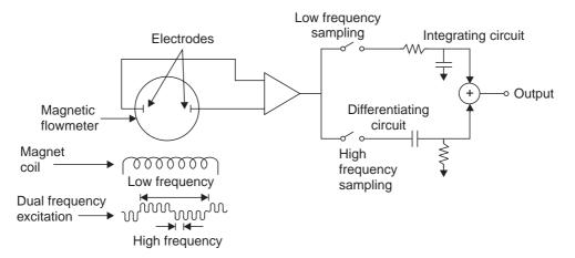
Fig. 1.55 Dual-frequency excitation Design
