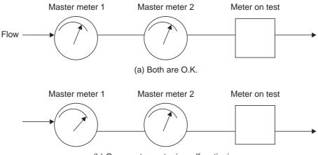
(b) One master meter is malfunctioning
