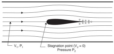
Fig. 1.20 Flow around a solid body
