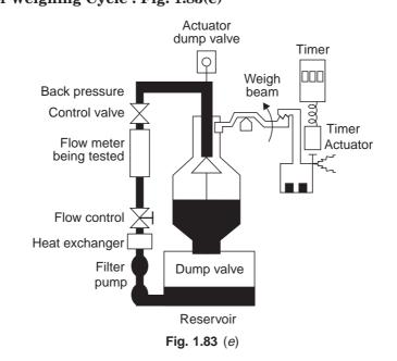
As the tank fills, the weigh pan rises, until it again trips the timer actuator, stopping the timer and the indicating the time within a thousandth of a second. By combining the precision test weight with the timed interval, the actual flow rate in kg/hr is easily and accurately determined. From these basic mass units, other flow units can be accurately calculated.
