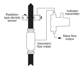
Fig. 1.50 Combination mass flow system
