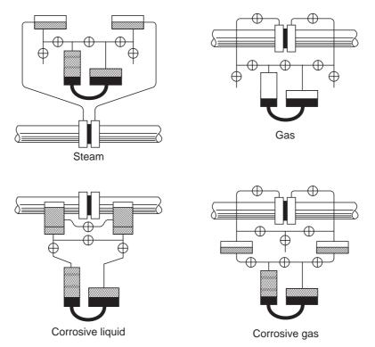
Fig. 1.19 Installation of Orifice Head meters
