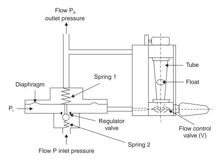
Fig. 1.63 Purge flow regulator consisting of a glass tube rotameter, and inlet needle valve, and a differential pressure regulator
