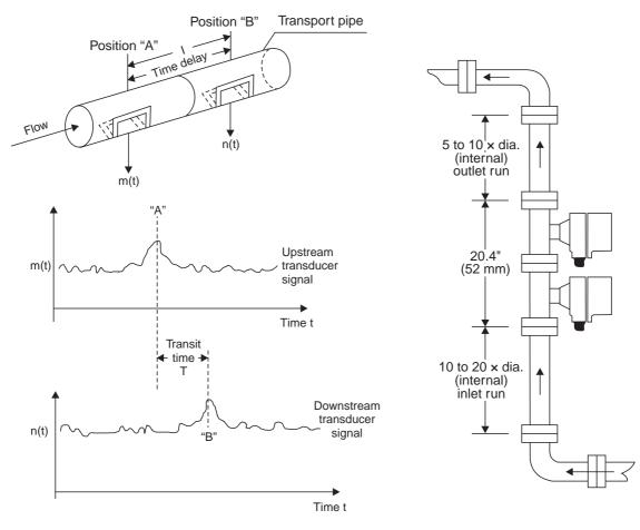
Fig. 1.64 Cross-correlation flow metering
