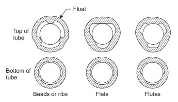
Fig. 1.37 Several types of glass rotameter tubes with ribs or beads for float guides
