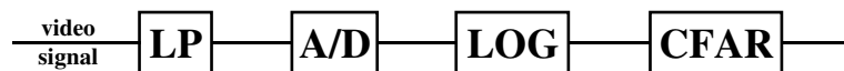
Figure 11.7 Signal processing chain for CFAR comparison (low-pass filter (LP), analog-to-digital converter (A/D) including magnitude calculation, logarithmic amplifier (LOG) and CFAR algorithm.
