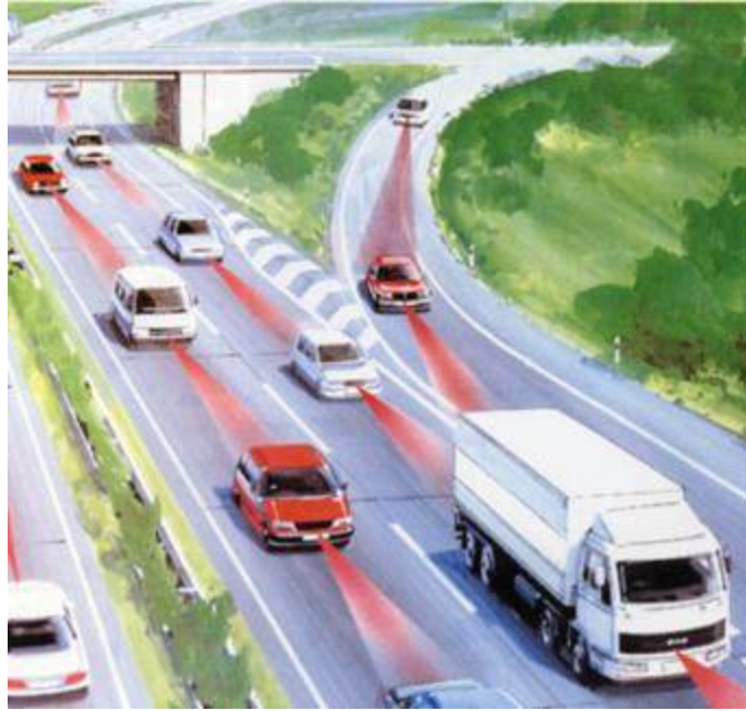
Figure 12.10 ACC radar sensors for highway and street traffic (Courtesy A.D.C.).
