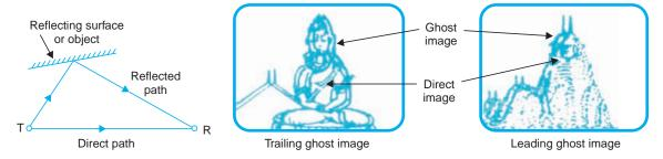
Fig. 9.4 (a). Geometry of multiple path transmission.
