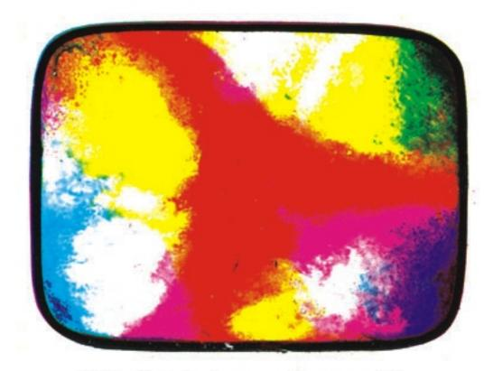
Colour Plate 6: Incorrect adjustment of the purity magnet
