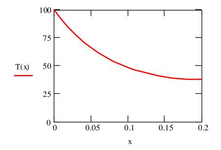
Temperature at the handle (x=0.2 m) is only 37.3 °C, not hot at all. This example illustrates the important role played by the thermal conductivity of the material in terms of conductive heat transfer.
