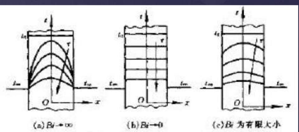
Problem: draw out the following temperature distributions according the situations, respectively.  $\lambda$  is constant. The right side of the body is insulated.
