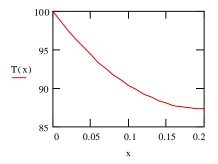
As shown, temperature drops off very quickly. At the midpoint  $T(0.1)=90.4^{\circ}C$ . At the end  $T(0.2)=87.3^{\circ}C$ . Therefore, it should not be safe to touch the end of the handle
