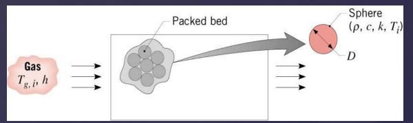
**KNOWN:** Diameter, density, specific heat and thermal conductivity of aluminum spheres used in packed bed thermal energy storage system. Convection coefficient and inlet gas temperature.
