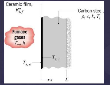
**KNOWN:** Thickness and properties of furnace wall. Thermal resistance of ceramic coating on surface of wall exposed to furnace gases. Initial wall temperature.
