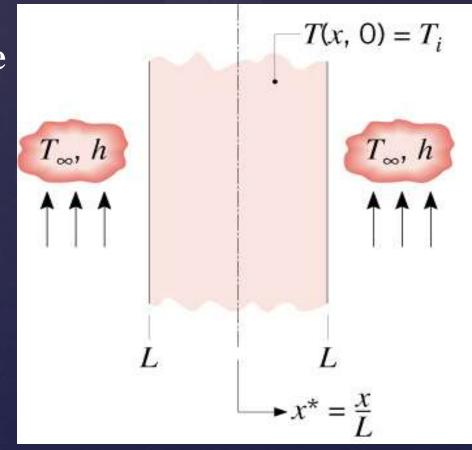
• For a plane wall with symmetrical convection conditions and constant properties, the heat equation and initial/boundary conditions are:
