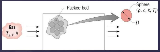
**KNOWN:** Diameter, density, specific heat and thermal conductivity of Pyrex spheres in packed bed thermal energy storage system. Convection coefficient and inlet gas temperature.
