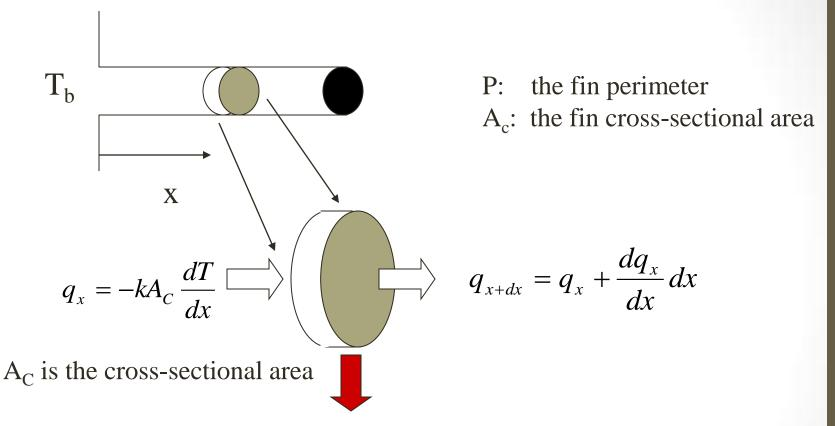
$dq_{conv} = h(dA_s)(T - T_{\infty})$ , where  $dA_s$  is the surface area of the element da
