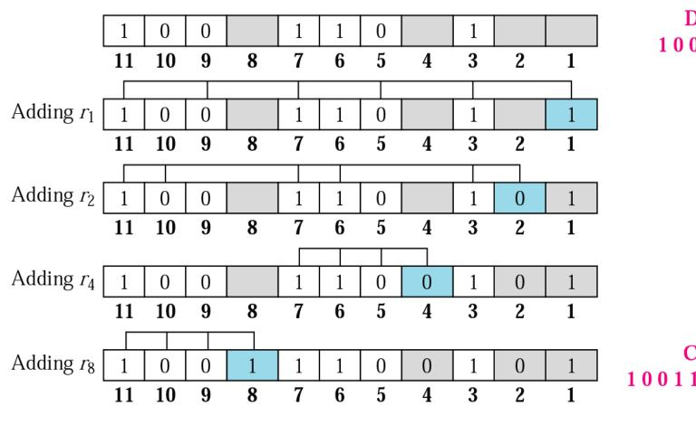
Error Detection using Hamming
