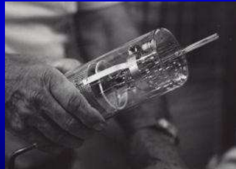
The Recreated Image Dissector, in the same hands that built the original 50 years earlier
