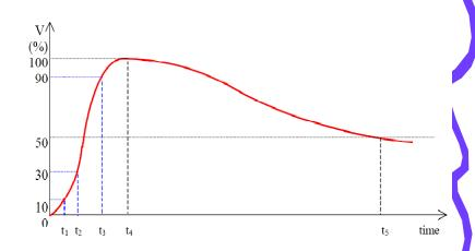
The wavefront time is given as  $(t_3 - t_1)/(0.9 - 0.1)$  or 1.25  $(t_3 - t_1)$  for the 10% to 90% measurement and as  $(t_3 - t_2)/(0.9 - 0.3)$  or 1.67  $(t_3 - t_2)$  for the 30% to 90% measurement.
