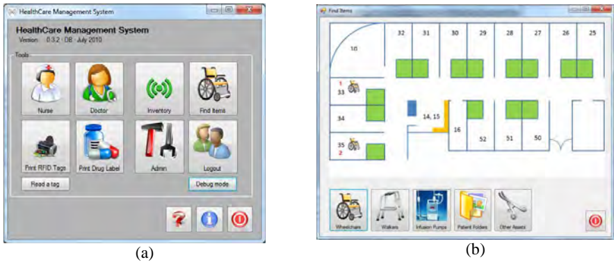
Fig. 4. (a) The Login card of the GUI; (b) The RTLS card where it is shown that 1 wheelchair was found in room 33 and 2 wheelchairs in room 35
