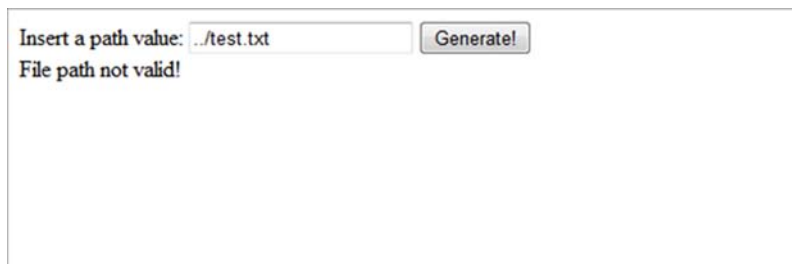
Figure 10.10 Path canonicalization is blocked by using our script in listing 10.6. This protection will ensure that malicious input is always blocked.
