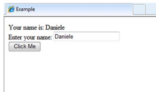
Figure 1.6 The code snippet results in a Web Form that shows the TextBox and Literal control after the button is clicked. The code used to render this page takes advantages of OOP techniques to program objects during their lifecycle.
