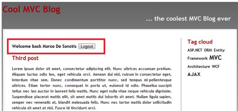
Figure 14.6 CoolMVCBlog provides a welcome message for the authenticated user. If we cached this whole page, the same message would be shown to everyone who visits our website.
