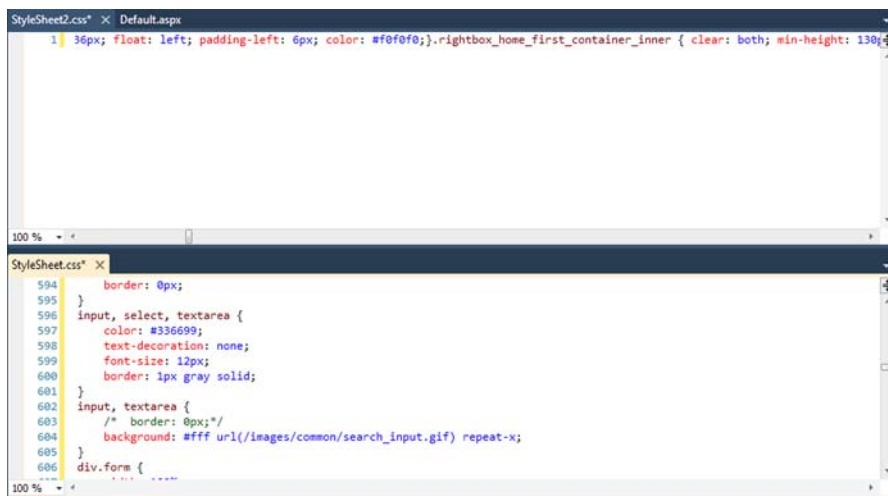
Figure 16.2 The minified version of a file (top) is composed of a single line, without spaces and tabs. The usual version contains a lot of unwanted characters.
