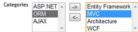
Figure 9.12 To modify the categories associated with a post, we use a custom editor that ASP.NET MVC cannot interpret with any built-in model binder.
